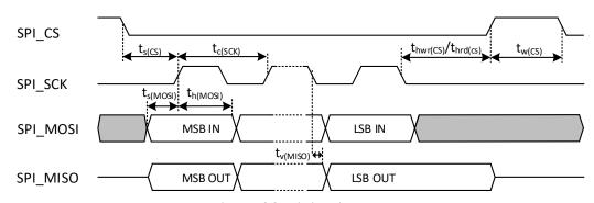
Figure 4-9 SPI Timing Diagram
