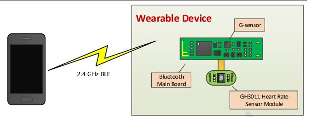
Figure 2-2 GH3011 Typical Application in Wristband
