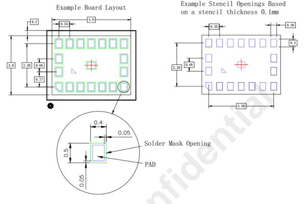
Figure 7-2 Package Design on PCB/FPC
