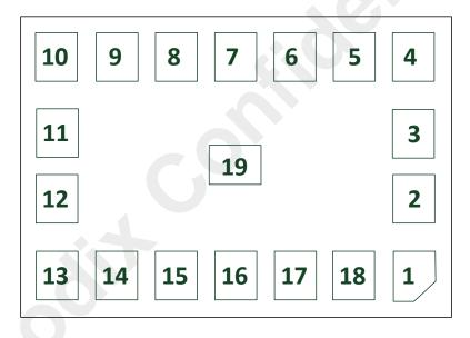
Figure 2-3 GH3011 Pin Assignment (Top View)
