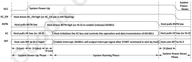
Figure 3-2 IIC System Control Timing Sequence
