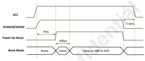
Figure 3-1 Power-Up/Down Timing Diagram
