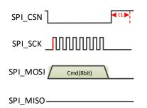
Figure 4-8 Data Format of SPI Command Issuance
