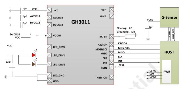
Figure 2-5 Sample Schematic for GH3011 Fingertip Oximeter Application
